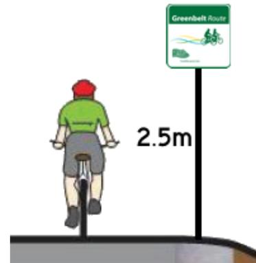
**Figure 3: Sign installation**
